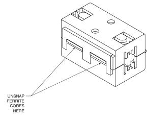
Figure 6-2 Ferrite Core
